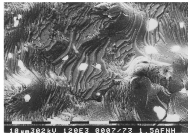
Fig. 3. Surface of an internally oxidized \text{Pd}_{0.985}\text{Al}_{0.015} at 1073 K (100%) showing faceted alumina precipitates (appearing white) and thermal grooves.
